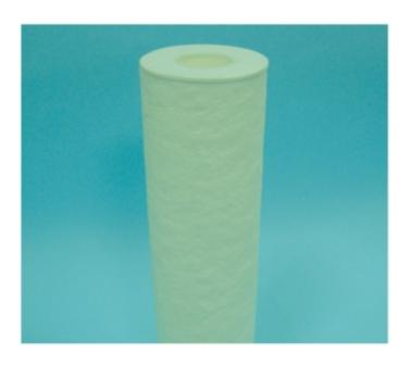
NPP Melt Blown Media Filter Cartridges are manufactured by a continuous spun-bonding technology that assures a consistent product. The 100% all polypropylene construction gives wide chemical compatibility and extremely low extractables. These cartridges offer exceptional value in both removal efficiency and dirt holding capacity where protection of more expensive membrane filters is important.
